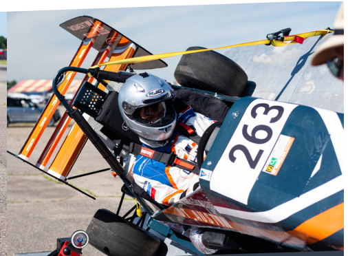
The Easy Driver undergoing the tilt test at competition
